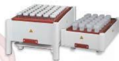
FluoroBloc FluoroPlate Inert tools for sample digestion
