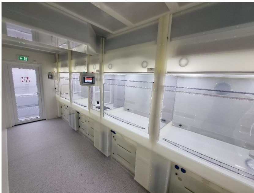
Fig. 1: View into an MK Mobile Lab with metal-free vertical laminar flow workstations
